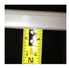
With the lid off, measure the protrusion of the lip of the bin. Be certain the bin has at least ½" of lip protruding beyond the exterior side of the bin.
