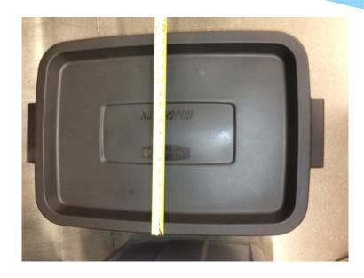
With the lid on, measure the overall width of the bin at widest point. Add ¼" to the total to determine the center-to-center spacing of the BinTRACKS. The bin shown measures 15% ¾" so when ¼" is added it suits standard 16" spacing.
